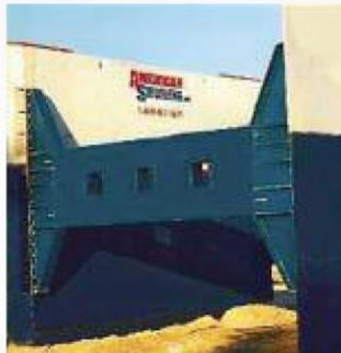
16' HIGH HEAVY DUTY BOLTED TRENCH BOX
