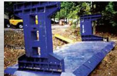
HEAVY DUTY BOLTED SPREADERS FEATURE "WINDOWS" FOR BETTER OPERATOR VIEWING. ADDITIONAL SPACERS CAN BE ADDED FOR WIDTH CHANGES
