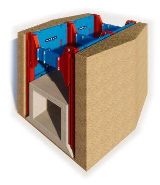
**2.** After placing the bottom support and respectively hardening the concrete slab, the rolling strut can be lifted up to the highest limit pin in the slide rail and fixed below using the limit pin.
